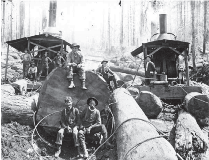
FIGURE 9. Lumber workers pose with “steam donkeys” in Washington State, probably around 1910. Charles R. Pratsch Photographs, Manuscripts, Archives, and Special Collections, Washington State University Libraries, PC 018.
